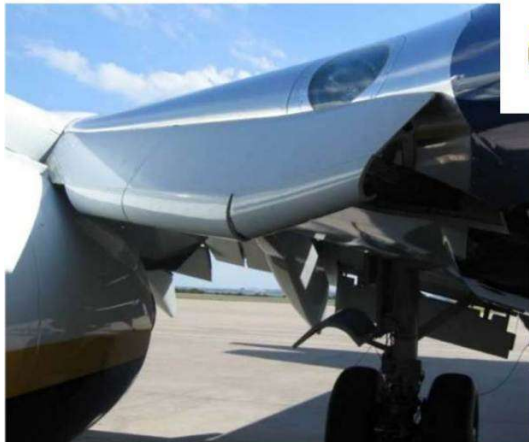
Leading edge Kruger flaps Extended Any time T.E. Flaps are not up.
